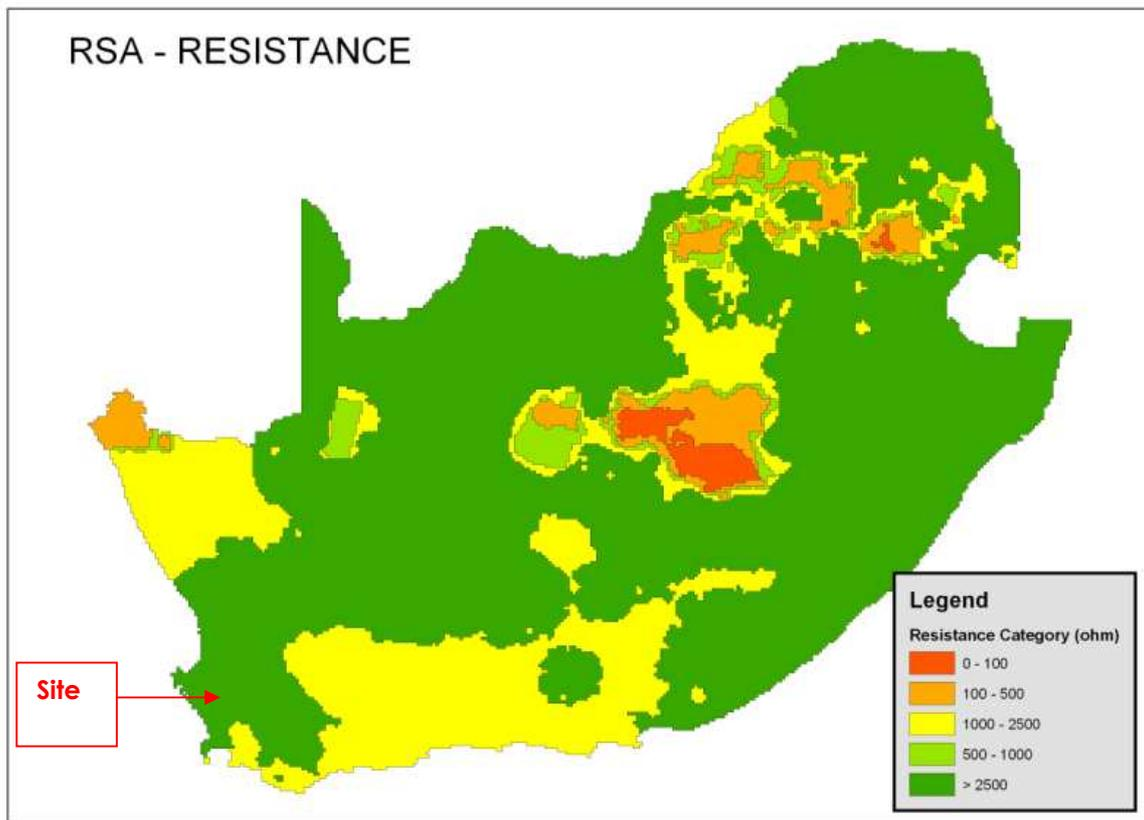
**Figure 6: Soil Resistivity Map - Koeberg Substation**
